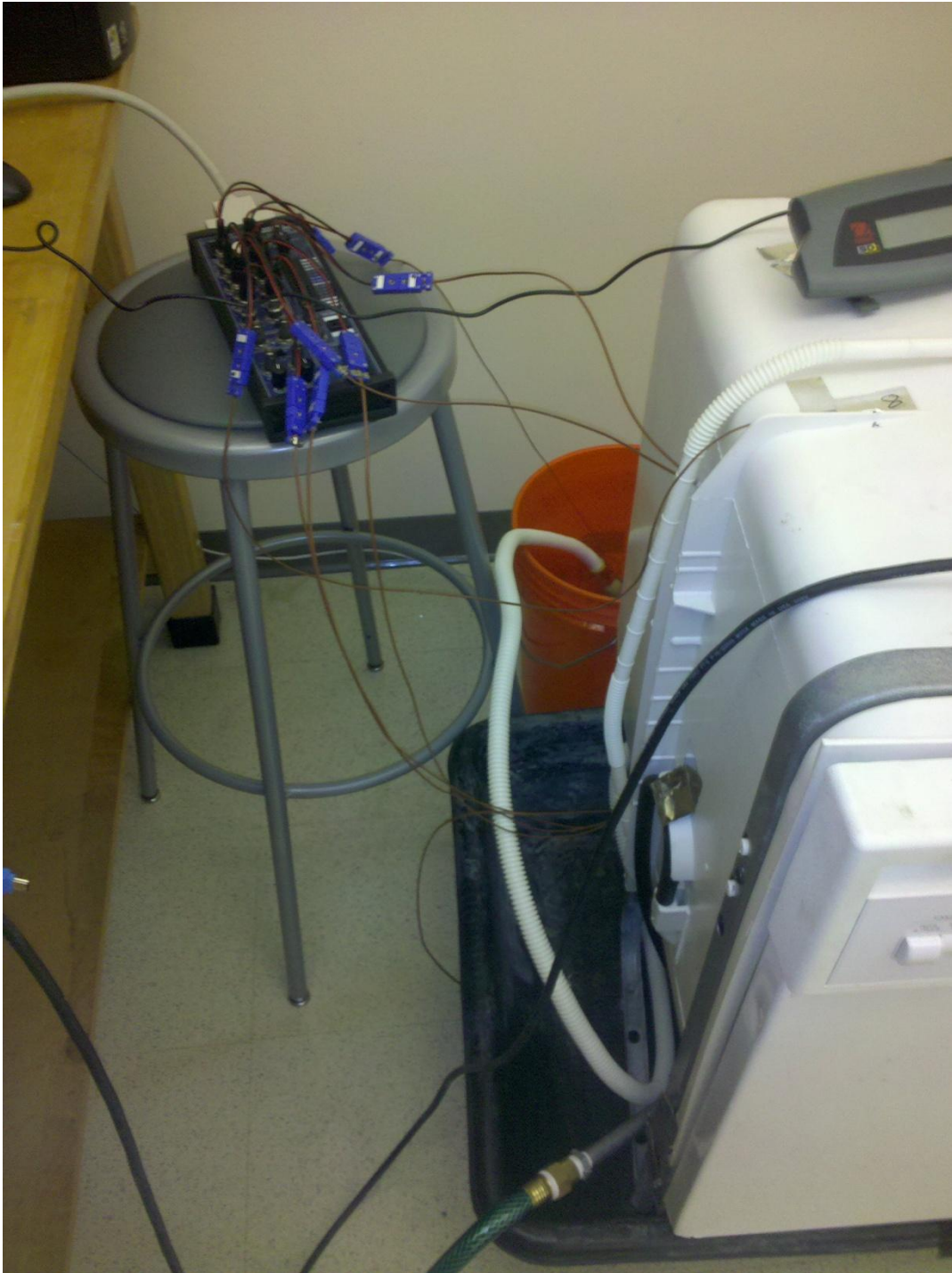
Figure 13: DAQ with Thermocouples Connected
