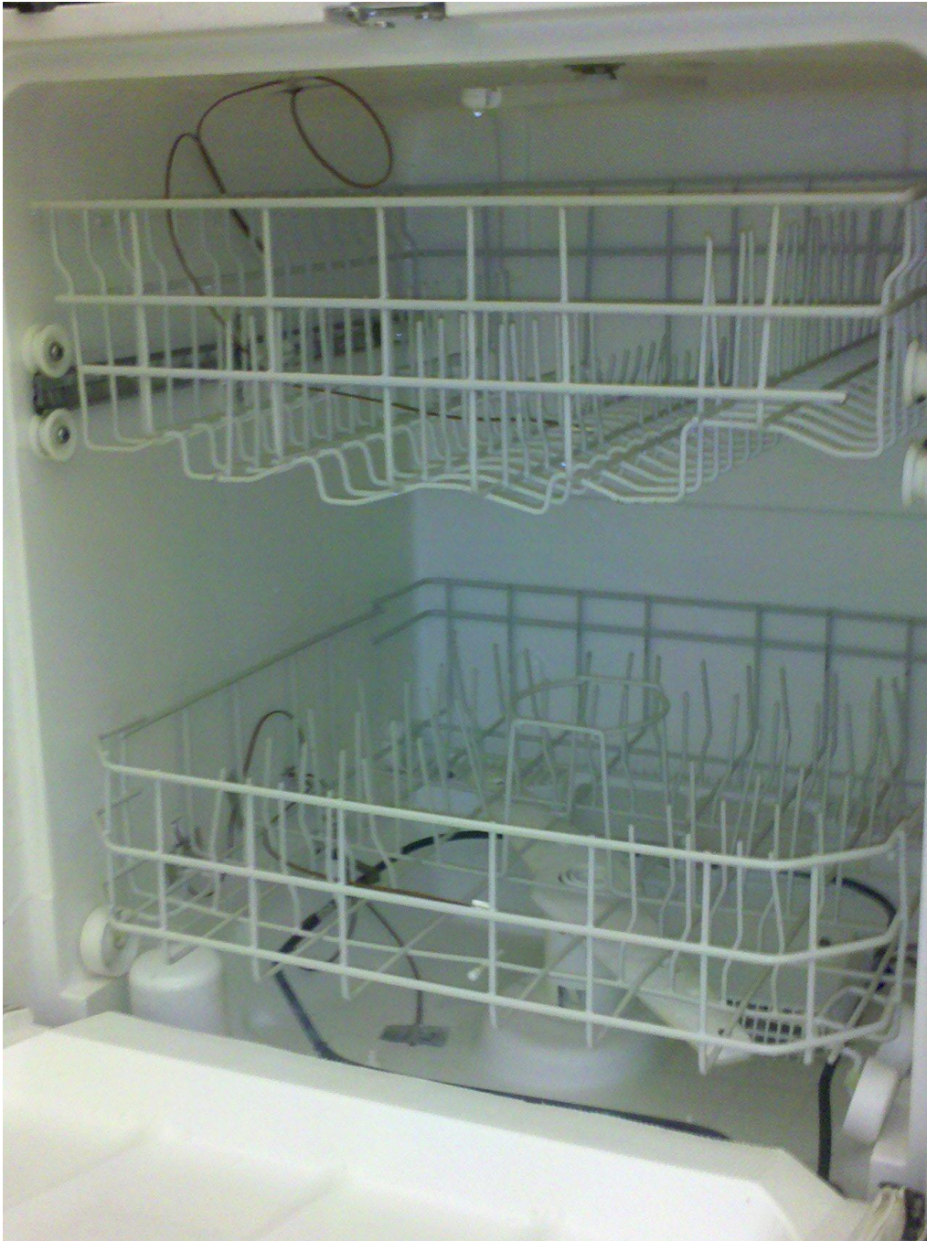
Figure 14: Internal View with Thermocouples
